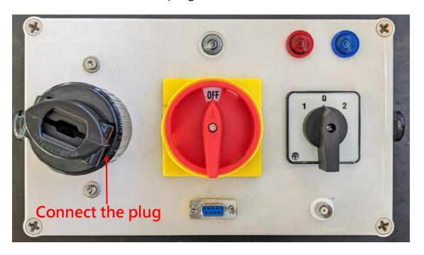
(3) Turn on the power switch. (Turn the red knob to the "ON" position.) After the unit is successfully powered on, a white LED will light up.
